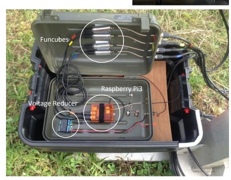
The mini-computer is a Raspberry Pi3, this is both the brain and the heart of the Motus installation. Finally there are three or four "Funcubes," these USB based radio receivers are the ears that monitor the antennas and produce the data that the Raspberry Pi records.
