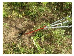
insufficient to wash bird excrement and other debris off of the solar panel. We have already had a case where a mammal dug a large hole immediately next to a guy line anchor.
