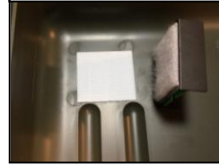
Figure 1: Affix Velcro to back of voltage converter and interior of case.
