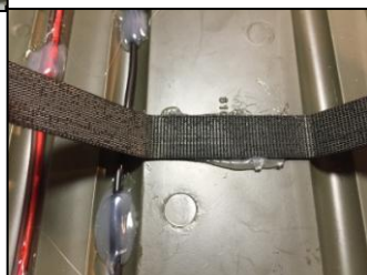
Figure 18: Once you determine where the Velcro strap will go, rough the location with sandpaper, make a line of glue, and press the strap in place it holds.
