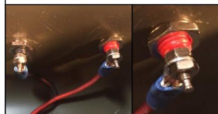
Figures 13: Tighten the inner nut against the post, then place eyelet, and secure with outer nut.
