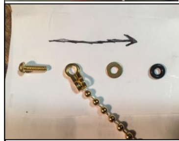
Figures 5 & 6: Secure the brass bolt with a nut inside the case. An O-ring against the exterior seals the drilled hole from water getting inside the case.
