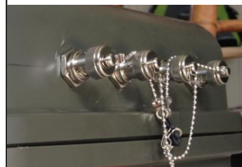
Figure 3: Connectors should fit in the hole snugly but go in easily. Widen the hole slightly with the drill, if necessary. Secure with nut and tighten with pliers.
