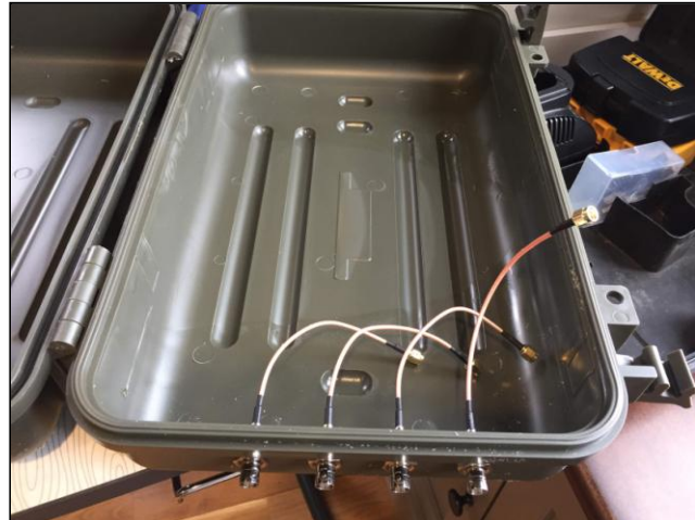
Figure 3: Connectors should fit in the hole snugly but go in easily. Widen the hole slightly with the drill, if necessary. Secure with nut and tighten with pliers.
